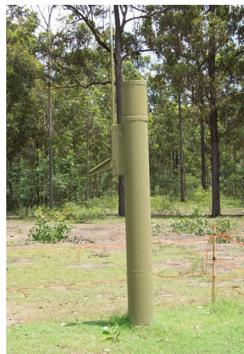
Automatic rainfall gauge.
